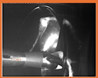
A comprehensive numerical and experimental survey has been conducted from NEWCASTLE UNIVERSITY, CNR, CHALMERS and DST to insight into the propulsive performance and the hydrodynamics of tubercle propellers. NEWCASTLE UNIVERSITY continued openwater testing of its newly designed propeller featuring tubercles, in the Emerson cavitation tunnel (emerson cavitation tunnel).
