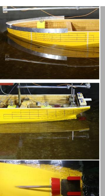
In June 2024 a first extensive model test campaign for the RESHIP inland vessel was completed at DST's large shallow water basin.
